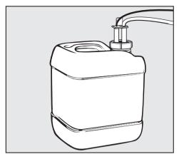
Insert and secure the siphon tube into the container. Observe the color code.
